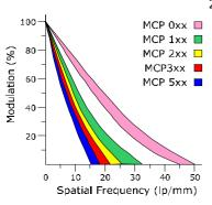
25 microns, which limits resolution to about 15 lp/mm. Our 12 mm tubes are built using 6 micron pore MCPs, which enables limiting resolution of 50 lp/mm, but 25 and 40 mm tubes are usually built with 10 micron pore MCPs giving resolution of 25-36 lp/mm.
