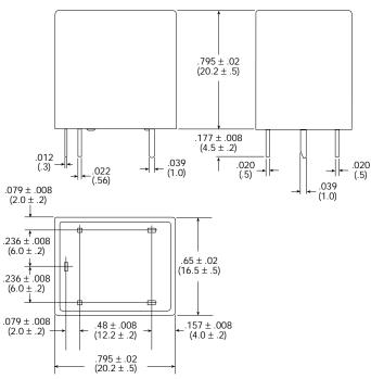
27E1064 socket is rated 10A @ 300VAC. UL Recognized for US and
