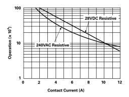
**Note:** This data is based on the max. allowable temperature for E type insulation coil (115°C).
