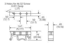
Note: Fits 35mm din track Includes: 2 Din clips 2 Screws Must be ordered in multiples of 50
