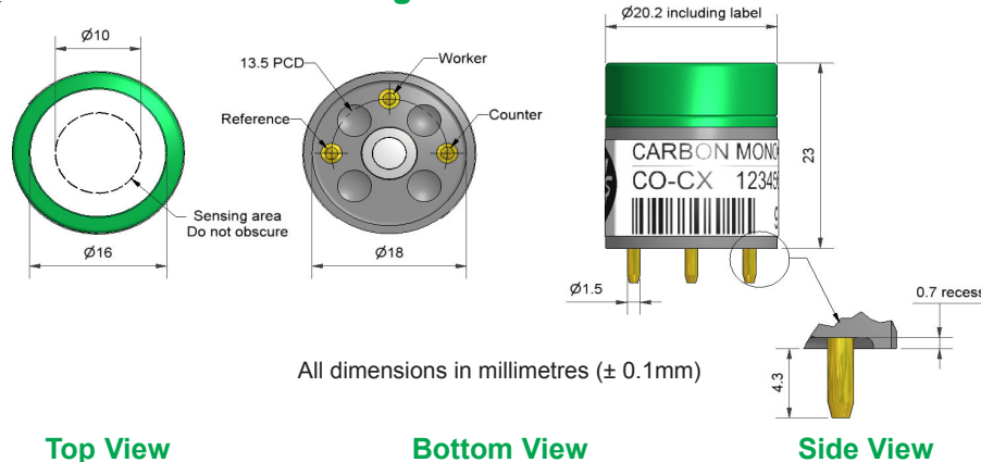
Figure 1 CO-CX Schematic Diagram
