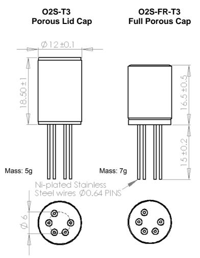
NOTE: Sensor pins are NOT designed to be solder too. Preferred method of connection is to crimp onto pins. All dimensions in mm.
