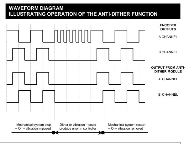
Note: For simplicity of illustration, the inverted channels, A/ and B/ have not been shown. The index, or Z, channel is also not shown in the above diagram but is passed through directly as an optically isolated signal and maintains its original relationship to the encoder output channel. Reference http://www.beiied.com/pdfs/oim.pdf for connection diagrams.
