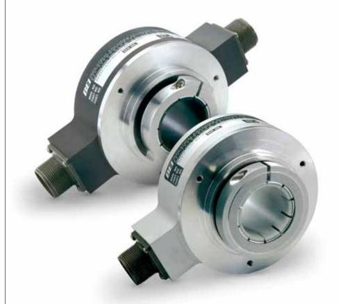
The HS45 is a large bore, heavy duty, rugged encoder designed to operate in very demanding environments. It is available in both single and dual output versions as shown above. These encoders use a preloaded bearing set for mechanical stability and a long service life. The dual output version has redundant electronics internal to the encoder simplifying signal distribution to multiple controllers.
