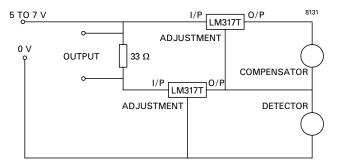
Note: Voltage across compensator and voltage across detector  $\simeq 1.25 \; \text{V}.$
