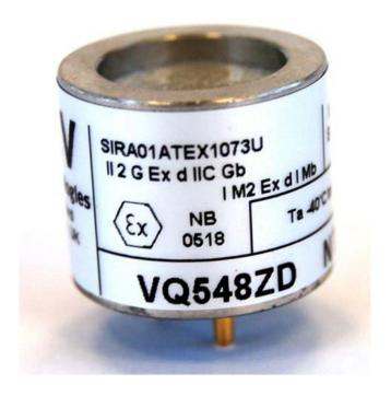
For the VQ548ZD/W, a carefully matched set of detector, compensator and resistor are encapsulated in a cylindrical stainless steel housing with an integral stainless steel sinter at one end to permit the entry of the atmosphere. Electrical connections are made to three pins at the other end of the body.
