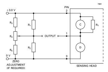
$R_1 = R_2 = 500\Omega$  to 10  $k\Omega$
