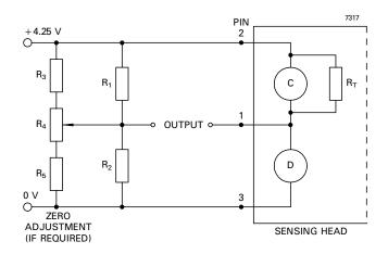
$R_1 = R_2 = 500 \Omega$  to 10  $k\Omega$   $R_3 = R_5 \simeq 10 R_1$
