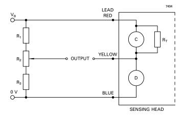
$R_1=R_3=500$  to 5000  $\Omega,~~R_2\simeq R_1/5$   $R_2$  provides zero adjustment and may be omitted if not required.
