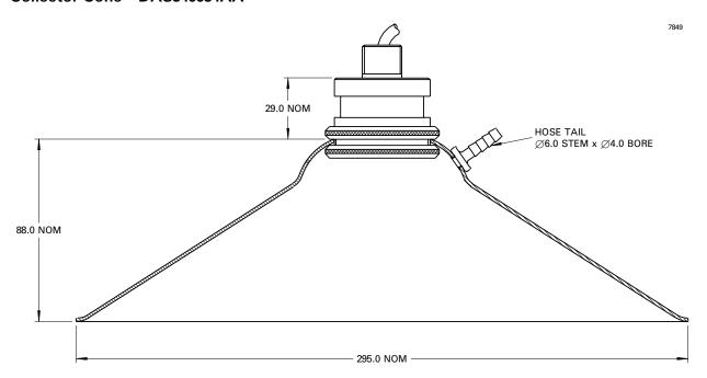
The Collector Cone is designed to enhance the performance of the VQ600 when used in applications involving the detection of leaks of gases which are lighter than air, such as hydrogen or methane. Easily fitted to the VQ600 via the external M46 thread, the assembly collects rising gases and directs them to the VQ600 for maximum detection sensitivity. The painted spun
