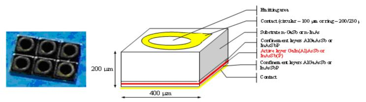
This shape of the LED chip is typical for most of IBSG standard Mid IR LEDs models.
