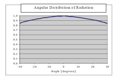
Some system designs cannot locate the detector plane very close to the emitter and a significant amount of energy falls outside of the detector collection "field of view".
