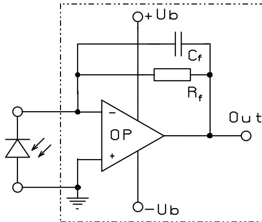
The application example shows a typical circuit..  $R_f$  is responsible for the gain of the circuit.  $C_f$  compensates the reverse junction capacitance of the photodiode and input capacitance of the OPV. The exact value of  $C_f$  depends on  $R_f$ , used OPV and capacitance of the circuit. A typical value is 1 pF.
