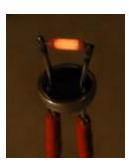
High electrical power consumption and low efficiency. Filter cuts only small part of wide emitted spectral range.
