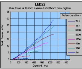
These characteristics are measured at repetition rate 500 Hz. 50% duty cycle corresponds to 1 ms pulse duration. Average vs. current and peak power vs. current characteristics for models: LED16, LED17, LED18, LED20, LED21 and LED23 are similar.
