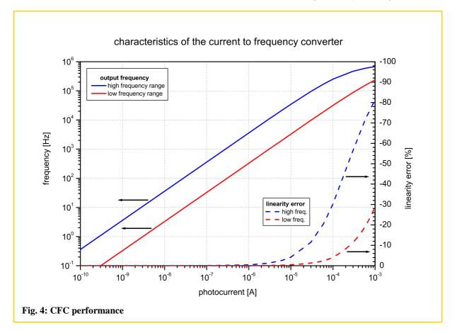
In programmable systems the linearity error can be corrected by using a matched lookup table. In this case frequencies up to 500 kHz can be used and thus the total dynamic range increases by two orders of magnitude.
