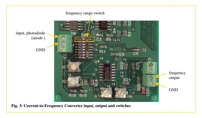
If there appears no pulse signal on the output, the polarity of the photodiode may be wrong. Also check that your equipment is able of recognising pulses as short as 1  $\mu$ s. Especially with older analog oscilloscopes and under artificial illumination it can be tricky to trigger these pulses because the output frequency may vary with the double of the mains frequency.
