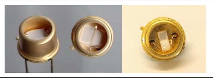
The IR source is based on a thin film which operates at approximately  $600^{\circ}$  (875K) when powered with 35 V for the IR-40 and 13V for the IR-43. The radiating element is a 1.5µm film of precision laser trimmed resistance material which has a high emissivity in the infra-red spectral region. The element is permanently bonded to a flat substrate of alumina forming a fixed and stable platform. This contributes to a uniform radiating source.
