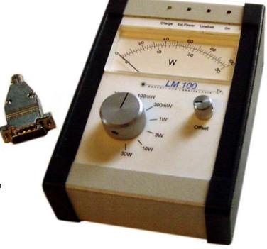
This read out unit is designed to measure the output power of different lasers in combination with a thermophile head. The maximum power is limited by the used power head. By using the read out unit it is possible to reduce the time constant of the whole measurement system to 1 second. Normally, the time constant of a power head is in the region of 15 to 25 seconds.
