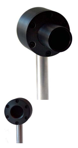
$\begin{array}{lll} \mbox{Diameter of sensor area} & 20 \mbox{ mm} \\ \mbox{Sensitivity} & 5 \mbox{ V/W} \\ \mbox{Time constant} & < 2 \mbox{ sec.} \\ \mbox{max. average power} & 3 \mbox{W} \\ \mbox{Detection threshold} & 10 \mbox{ } \mu \mbox{W} \\ \mbox{max. power density} & 2,5 \mbox{ W/cm}^2 \end{array}$
