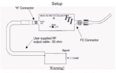
No voltage should be present at user interface or damage to the unit may occur.
