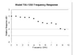
The TIA-1200 is comprised of a fiber coupled InGaAs detector coupled with a reverse bias voltage network. The ouput of the diode is brought out to a type K female SMA connector. Light falling on the detector generates a positive-going proportional current. This current, multiplied by the load impedance produces a voltage that is proportional to the light incident on the detector surface.
