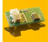
Other modules with low gain (AMPCON\_LO, up to 250µA) and high gain (AMPCON HI, up to 18nA) are available. Alternatively, please refer to the below instruction for changing the gain.
