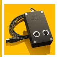
The DIGIBOX is a CAN to USB converter box converting the CAN output signal of the digital sglux UV sensors into an USB signal. Up to eight sensors can be connected to the box
