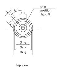
UVB-only SiC based UV photodiode A = 0,50 mm<sup>2</sup>
