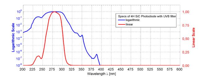
UVB-only SiC based UV photodiode A = 0,50 mm<sup>2</sup>
