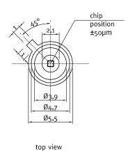
UVC-only SiC based UV photodiode A = 0,50 mm<sup>2</sup>
