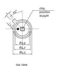
Broadband SiC based UV photodiode A =1,0 mm<sup>2</sup>
