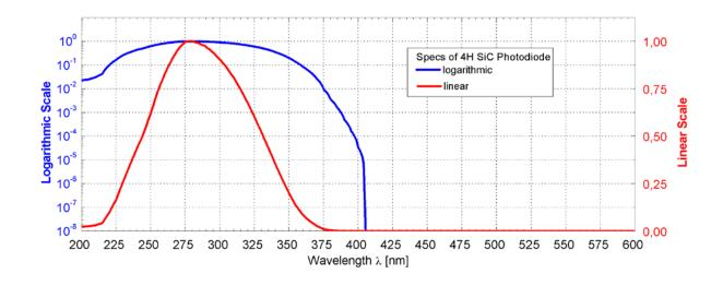
Broadband SiC based UV photodiode A = 0,20 mm<sup>2</sup>
