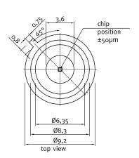
UVA-only SiC based UV photodiode A = 0,20 mm<sup>2</sup>
