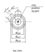
UVB-only SiC based UV photodiode A = 0,20 mm<sup>2</sup>
