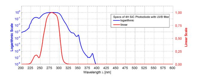
UVB-only SiC based UV photodiode A = 0,20 mm<sup>2</sup>
