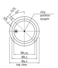
Broadband SiC based UV photodiode A = 0,06 mm<sup>2</sup>
