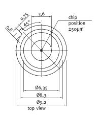
UVC-only SiC based UV photodiode A = 0.06 mm<sup>2</sup>
