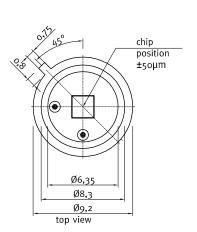
Broadband SiC based UV photodiode A =4,0 mm<sup>2</sup>
