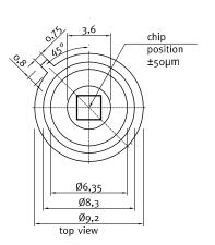
UVA-only SiC based UV photodiode A = 4,0 mm<sup>2</sup>
