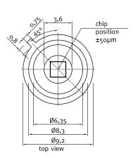
UVB-only SiC based UV photodiode A = 4,0 mm<sup>2</sup>
