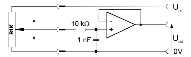
For applications with higher input currents, we recommend our integrated signal processing options 10V, 420A, 420T, PMUx with 0-10V or 4-20mA outputs. Alternatively, ASM offers external signal processing modules, WS-UMR-10V and WS-UMR-420A, that were especially designed for ASM sensors with hybrid potentiometers and are guaranteed to provide the best linearity and longest life expectancy.
