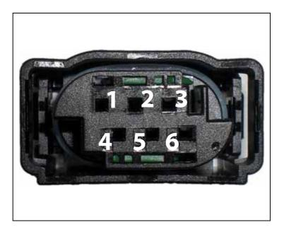
Figure 6: Pin Assignment
