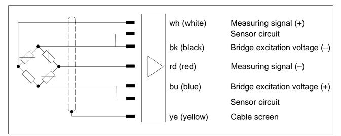
Fig. 7.2: Transducer with four-core cable, amplifier in six wire technique
