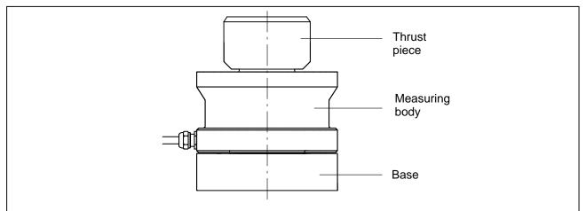
Fig. 5.1: Schematic diagram of the force transducer
