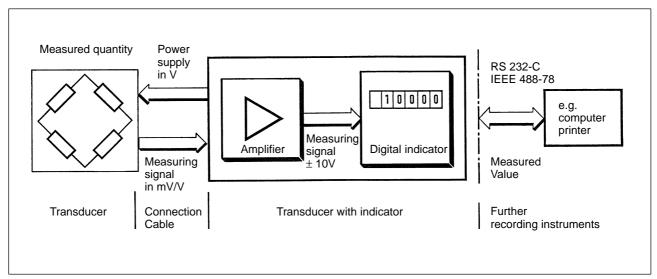
Fig. 6.1: Basic diagram of measuring system
