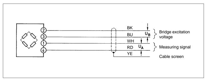
Fig. 7.1: Transducer with four-core cable
