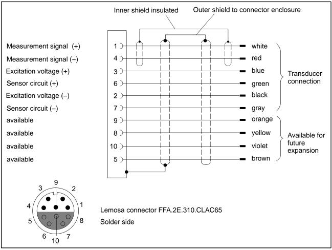
Abb. 4.1: Electrical connection of the P3MBP pressure transducer
