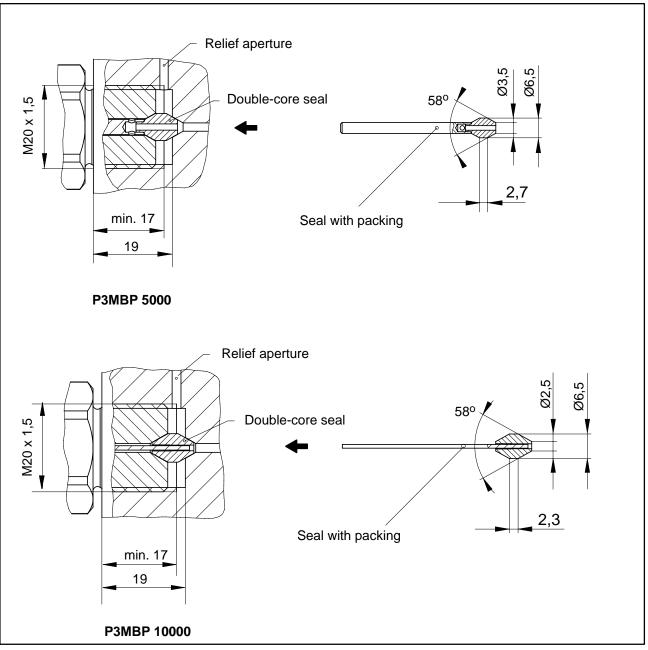
Fig. 3.1: Installing the pressure transducer
