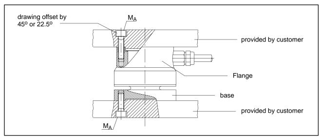
Fig. 5.3 Installation for compressive loading
