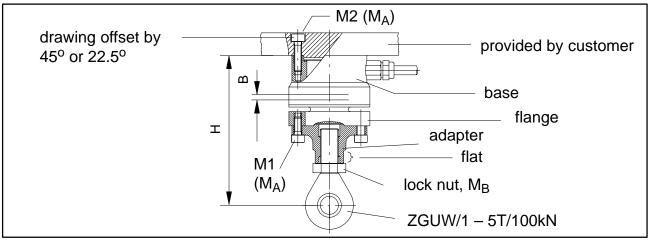
Fig. 5.4 Installation for tensile loading
