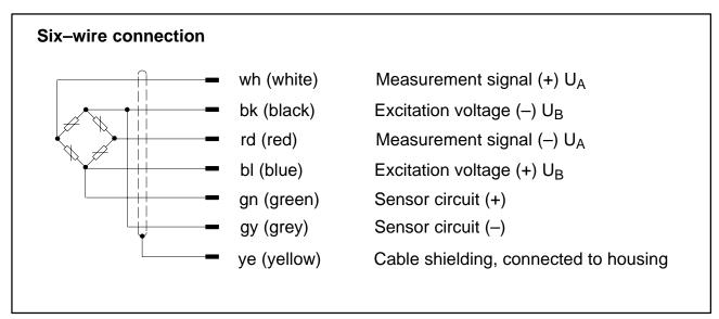
Fig. 6.2: Pin assignment for the U3
