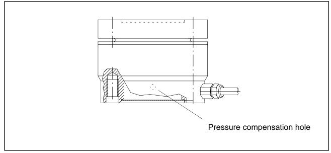
Fig. 3.1 Position of housing base
