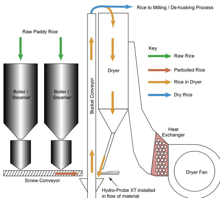
**Figure 1: Hydro-Probe XT moisture sensor installed after dryer**
