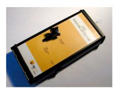
The **UVC Photon Detector** is designed to measure very low UVC radiation intensities. It is a useful instrument where harmful UVC radiation needs to be detected or other applications where a UV photodiode is not sensible enough. Once installed in the laboratory the unit alarms if invisible UVC radiation is present.
