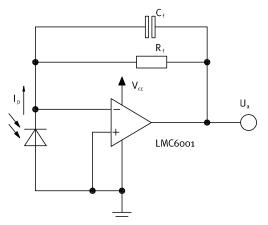
Calculations and Limits:  $U_a = I_p x \ R_f = \ o \ ... \ \sim \ V_{cc}$
