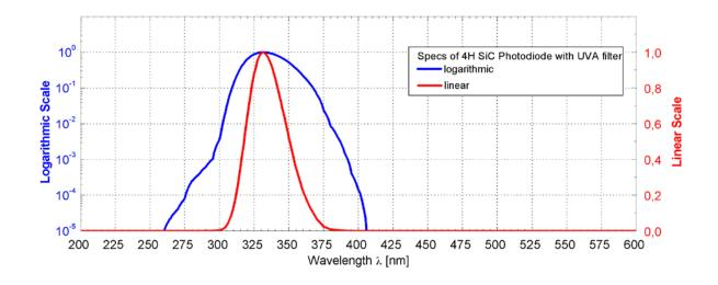
UVA-only SiC based UV photodiode A = 1,0 mm<sup>2</sup>
