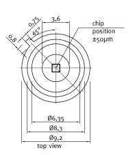
UVA-only SiC based UV photodiode A = 1,0 mm<sup>2</sup>
