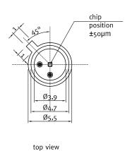
Broadband SiC based UV photodiode A = 0,20 mm<sup>2</sup>
