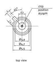
UVA-only SiC based UV photodiode A = 0,20 mm<sup>2</sup>
