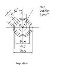
UVA-only SiC based UV photodiode A = 0.06 mm<sup>2</sup>
