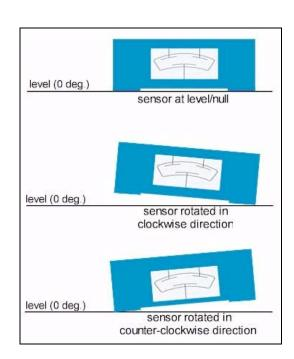
Turn 'Sensor Null Adjustment' potentiometer until output on Digital Voltmeter reads 0.000Vdc (see below for potentiometer locations).
